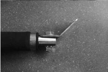
Check that the screw connecting the shoe to the cable lug is tight.
