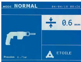
In normal mode, the gun will be limited to 1.5mm thick sheets. Using the gun, the operator can choose between different tools (mono point, star, impact, heat, dowel pin, rivet, nut, toothed wheel). Select the desired tool using the + and - keys.
