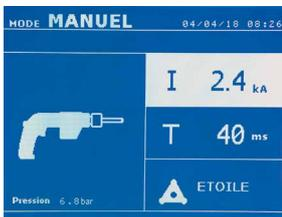
In Manual mode, the maximum possible intensity is 8 kA for a maximum duration of 500 ms. The settings showing on the screen will not exceed these values. Set the generator by indicating the thickness of the sheet/panel to weld using + and - keys. It is possible to adjust the current and time settings when in manual mode.
