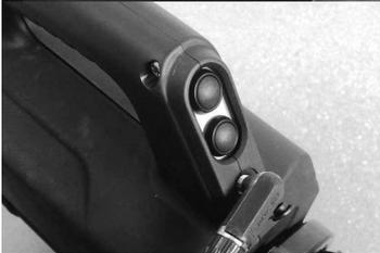
Connect the control cable to the jack plug.
