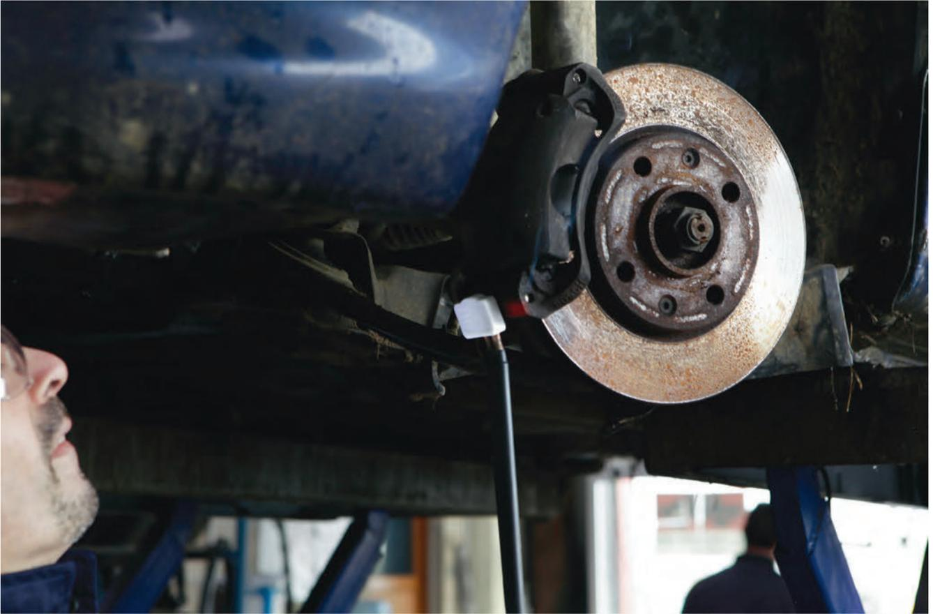
**G**YS, the best-known manufacturer of car body repair equipment and battery chargers, has developed a range of powerful induction heaters. For decades, getting metal to expand has been done using a flame torch. Not anymore. Induction is the revolutionary method of heating metal by using electromagnetic fields. Heating from the inside out, this flameless process is much quicker, safer, and more precise than naked flame.
