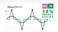
The GYSMI E200 FV has a powerful integrated PFC and features FLEXIBLE VOLTAGE (85-265V).
