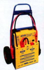
This mobile battery booster pack delivers a maximum 6,200A for a 12V battery and 3,100A for a 24V battery. This pack when fully charged is sufficient to start up to 28 trucks with 12V batteries or 16 start ups on 24V batteries between re-charging.
