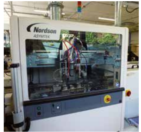
The production workshop for electronic cards is now equipped with a new coating machine, which protects against build up of dust and corrosion; an important factor in areas with high humidity.
