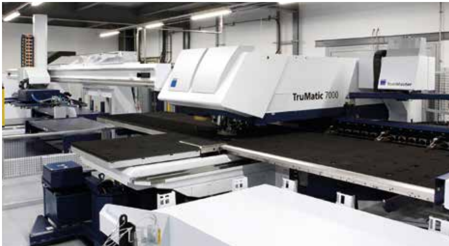
Amongst recent investments is a new sheet metal cutting machine. The new machine has the ability to undertake punching and laser cutting operations allowing work with thicker materials with increased cutting quality in a shorter period of time.
